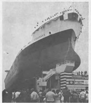
Poised high and ready to enter the sea is the S/S Coronado, 38,300-dwt Coronado Class tanker, being built at NASSCO for Margate Shipping Company. The new ship is 688 feet in length, 90 feet in beam, and has a 47-foot molded depth.
