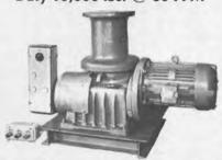
MOTOR: 10 HP—totally enclosed—fan cooled—continuous duty—horizontal flange mounted—special shaft & oil seal fitted—440/3/60—1760 RPM. CONTROL: Marine type watertight pushbutton—forward / reverse / stop—watertight starter box—rated for 40 starts/hour—triple pole contactor with silver contacts, thermal overload relay & trip adjustment. DIMENSIONS: Barrel 10" diam.—flange 10" diam.—approx. 26" wide & 36" long.
