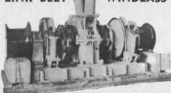
Below deck motor drive. Double wildcat—driven by 50 HP 230 VDC motor with vertical shaft and worm drive. Single speed—handles 7000 lb anchors and 60 fathoms of 15/8" chain at 7 fathoms per minute. Wildcat centers 56". Complete with all controls and warping features. Total weight 27,500 lbs. With spares.
