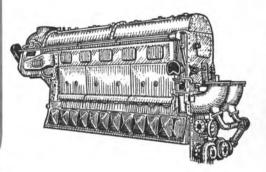
MATCHED PAIR . . . FAIRBANKS-MORSE Model 38D8-1/6—1 Port; 1 Starboard. Used condition, 1800 HP, 800 RPM, 2 cycle, 81/2" bore, 10" stroke, Air Start. Complete with Westinghouse Reduction Gears, 2.216:1 ration—with Hydraulic Coupling.
