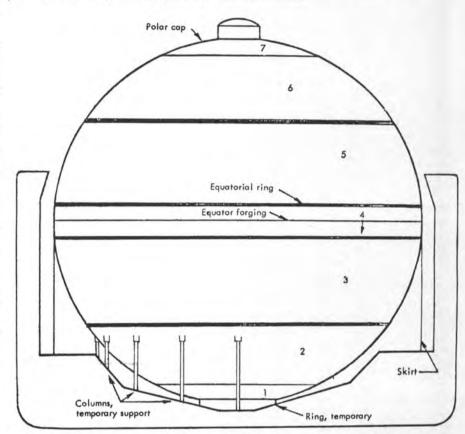
TANK ASSEMBLY sketch shows the seven separate tank sections and method of erection.
