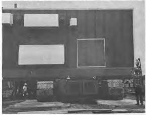
A large low-profile "creepy crawler" moves under the 559-ton camp module (also shown in top picture). The crawler hydraulically lifts the heavy modules up and slowly moves them aboard the barges.
