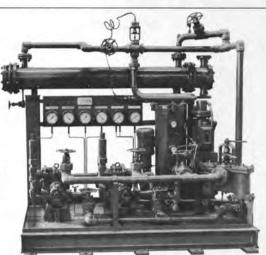
Auxiliary lube oil system for marine use designed and manufactured by Modular Systems
