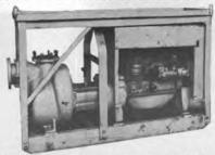
Reconditioned—mounted in portable steel frame, 1750 RPM—1100 GPM @ 100' head; 1500 GPM @ 70' head; 1800 GPM @ 50' head; 2100 GPM @ 20' head. Leroi gas engine—model D-201P3
