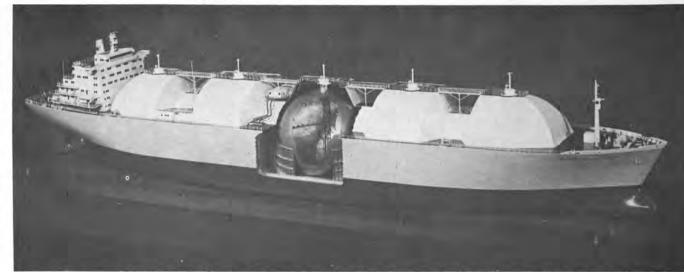
Model of the 87,600-cubic-meter ship with cutaway in the cargo tank area. Built of 9 percent nickel steel, each of two of the tanks have a diameter of 101 feet 7 inches, and the other three have diameters of 108 feet 3 inches.
