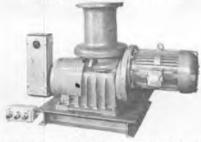
MOTOR: 10 HP—totally enclosed—fan cooled—continuous duty—horizontal flange mounted—special shaft & oil seal fitted—220/440/3/60—1760 RPM. CONTROL: Marine type watertight pushbutton—forward / reverse / stop—watertight starter box—rated for 40 starts/hour—triple pole contactor with silver contacts, thermal overload relay & trip adjustment. DIMENSIONS: Barrel 10" diam.—flange 10" diam.—approx. 26" wide & 36" long.
