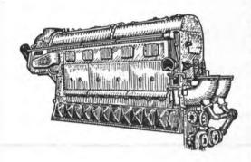
MATCHED PAIR . . . FAIRBANKS MORSE MODEL 38D8-1/8—1 Port; 1 Starboard. Used condition, 1800 HP, 800 RPM, 2 cycle, 8 ½" bore, 10" stroke, Air Start. Complete with Westinghouse Reduction Gears, 2.216:1 ratio—with Hydraulic Coupling.
