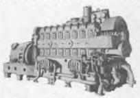
ENGINE: 8-268A—61/2" bore x 7" stroke—1200 RPM—driving 200 KW Westinghouse generator—440 volts—3-phase—60 cycle—321 amps—80% power factor at 1200
