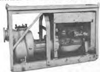
Reconditioned—mounted in portable steel frame. 1750 RPM—1100 GPM @ 100' head; 1500 GPM @ 70' head; 1800 GPM @ 20' head; 2100 GPM @ 20' head. Leroi gas engine—model D-201P3
