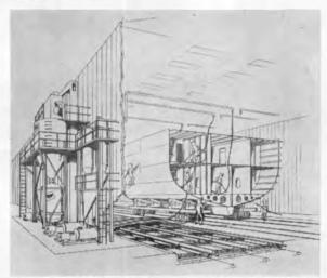
The system for blasting and coating is housed in a totally enclosed building. The abrasive material is reclaimed and readied for re-use in 90 seconds, all mechanically.
