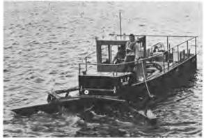
The DIP skimmers have the ability to harvest any floating material, including debris and sorbents, without changing the skimmer configuration.
