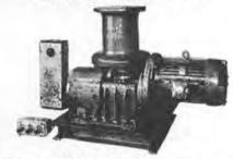
10 H.P.-220/440/3/60-1750 R.P.M.-Marine type reversing controller. Barrel diameter-10"-21/2" Flange. Height between flanges 12".
