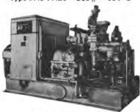
We offer with ABS or Lloyd's certificate. Our reconditioning of this unit is fully guaranteed on a money-back basis. Has been through G.E. Engineering and the last stage has been rebladed with new style blading. All diaphragms re-machined.
