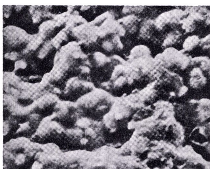
ANTI-FOULING DYNAMIC magnified 8000 times by Scanning Electron Microscope. By permission of The Danish Technological Institute, Copenhagen.
