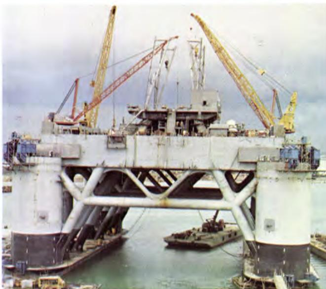
**REPUBLIC OF SINGAPORE** *Margie*, semisubmersible, twin hull, measures 202' long x 182' wide x 110' high; 9,000 tons. Designed to drill in 600' of water. Crew of 90. Scheduled to drill off the coast of Northern Australia.
