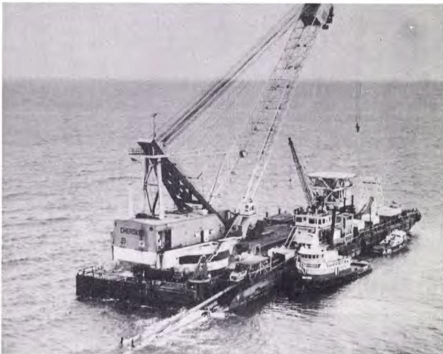
SANTA FE INTERNATIONAL'S CHEROKEE, converted to work as bury barge on Ekofisk pipeline, has eight 4,000 BHP Alcos driving high pressure water pump to bury sled.
