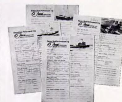
**RECORD AND PERFORMANCE LOGS** of all Demountable-fitted vessels go to 30 Johnson Reps around the world, and are regularly updated. Data includes vessel name, a photo, bearing locations and dimensions, drawing references—everything needed to expedite service at any repair yard. Copies go to ship's files. If you'd like to see some typical ones, drop us a note.
