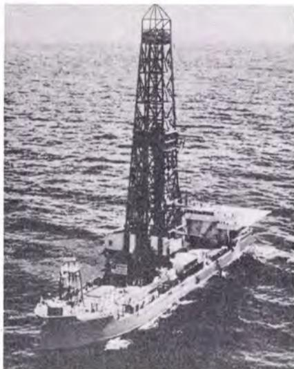
Three ALCO, 12-cylinder diesels power drill ship DISCOVERER II in Malaysia.
