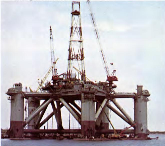
**CLYDEBANK, SCOTLAND** *Penrod 64*, jackup, hull dimensions of 230' x 200' x 26'; 6,000 tons. Designed for TD of 30,000'. Crew of 78. Scheduled to operate in North Sea.
