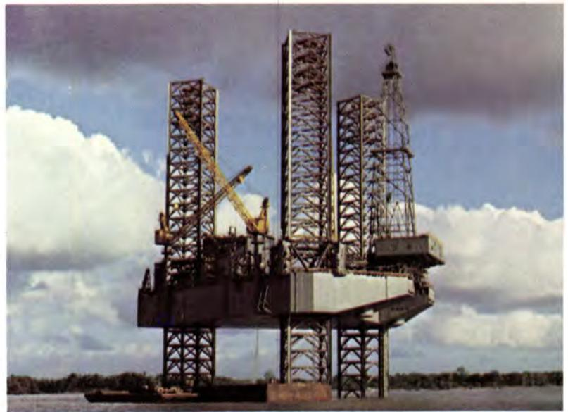
**VICKSBURG, MISSISSIPPI** *Key West*, jackup, 230' long, 200' wide, legs 467' high; 6,000 tons. Designed to drill in 300' of water. Crew of 97. Notice the three 45-ton marine cranes, usually on almost all rigs Marathon constructs. Scheduled to drill in waters off Belem, Brazil.
