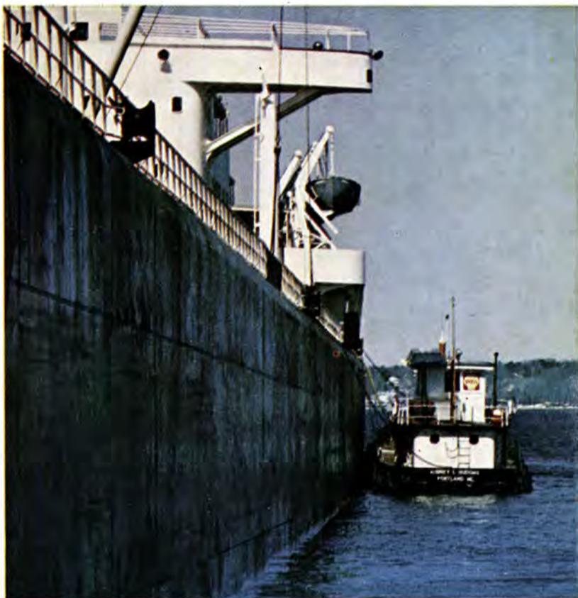
Golden Ship Repair tank boat, the Aubrey L. Hudgins, pumps Shell MELINA Oil into ship in mid-harbor at Portland, Maine. The Hudgins' pumps can deliver 4,800 gallons per hour from her 48,000-gallon-capacity tanks. Turnaround time for ships is speeded up by this fast, clean delivery system.
