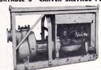
Reconditioned—mounted in portable steel frame. 1750 RPM—1100 GPM @ 100' head; 1500 GPM @ 70' head; 1800 GPM @ 20' head; Leroi gas engine—model D-201P3
