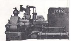
TURBINE: 11 Stage type FN4— 8145 RPM—31/2" absolute back pressure—complete steam with seal regu GEAR: Type S-195A-reduction 8145 RPM to 1200
