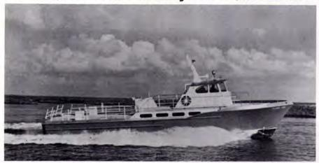
**ON THE COVER:** The Gacship IV is powered by three Caterpillar D-343 turbocharged after-cooled engines and can reach a speed of 23 mph.
