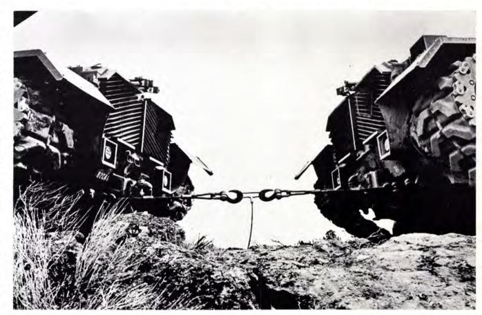
We put three different swaged sleeves through the toughest torture test we could devise: a side-pull test designed to tear wire rope slings apart at the sleeves. This is what happened: In a tug of war between two 52-ton tanks, the  $V_2$  " aluminum and carbon sleeves ripped apart, but the ESCO  $V_2$ " stainless duplex sleeve wouldn't give up.
