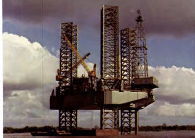
VICKSBURG, MISSISSIPPI Key West, jackup, 230' long, 200' wide, legs 467' high; 6,000 tons. Designed to drill in 300' of water. Crew of 97. Notice the three 45-ton marine cranes, usually on almost all rigs Marathon constructs. Scheduled to drill in waters off Belem, Brazil.
