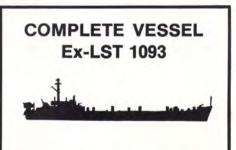
Steel hull, twin screw, 1800 HP, 328' length overall, 50' beam, 14' draft, light displacement 2100 tons.
