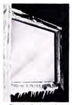
Electrically heated Kearlott window exposed to 45 knot gale, -20° spray.
