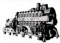
ENGINE: 8-268A—6½" bore x 7" stroke—1200 RPM—driving 200 KW Westinghouse generator—440 volts—3-phase—60 cycle—321 amps—80% power factor at 1200 RPM. Switchgear available.
