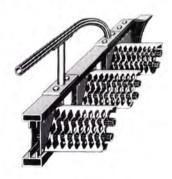
All models are 6061-T6 aluminum with a minimum yield of 38,000 p.s.i. All rungs are electrically welded to outer truss plates and internally expanded to inner truss plates. All models are on 12" centers (per OSHA) and feature all aluminum or plated steel fittings.
