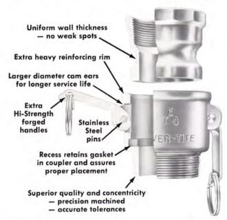
Sizes from  $\frac{1}{2}$ " to 10". Choice of metals, gaskets, male or female NPT or straight threads, hose shanks, flanges, or machined for socket or butt weld. Also valved couplings to connect or disconnect *full* lines without spillage.
