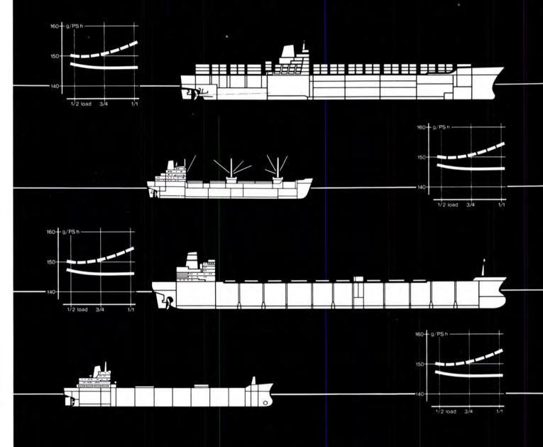
By further developing the injection and gine, M.A.N. have cut its fuel consumption rate by 8g/HPh. Sample calculation: Standard freighter ម៉ឺ with 16V 52/55A
