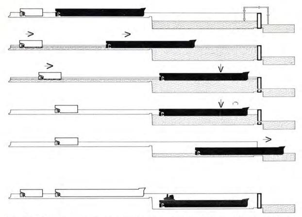
Schematic plan for launching a new vessel. The top view shows the completed new vessel plus the stern section of another ship under construction. The bottom view shows the facility in use for both new construction and repairs. The new construction platform, at left, is on the shipyard ground level.
