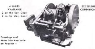
Watertight Construction. Complete unit is of non-magnetic construction (S.S. Drum, etc.) Automatic spooling device. Drum free spool up to 500 f.p.m. Drum provided with a dog capable of withstanding the breaking strength of the cable. Also this dog is electrically interlocked with the control, to prevent operation of the motor while dog is applied.
