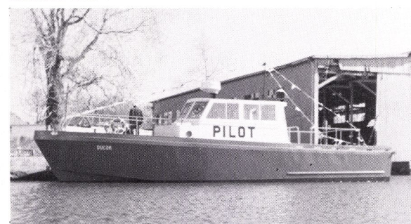
The all-welded steel pilot boat Ducor is powered by twin Detroit Diesel model 8V-71 engines.
