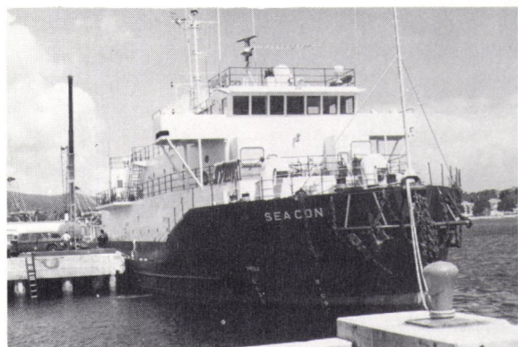
Converted at Norfolk Shipbuilding and Drydock's Berkley Plant, the SEACON, with 6,240 square feet of open deck aft, can be rigged for a variety of offshore construction tasks. (Official U.S. Navy photo)
