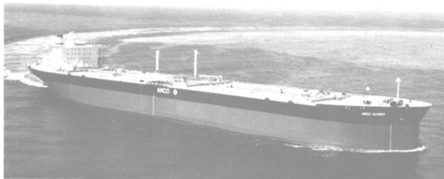
The ARCO Alaska, 188,500-dwt San Diego-class tanker, built by NASSCO for Arch Tankers, Inc.
