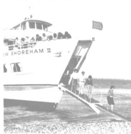
Unique Bow Ramp (patent pending) designed by Luther Blount allows visits to many unspoiled and previously inaccessible areas.
