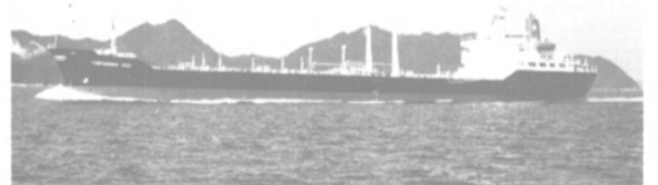
Powered by a Hitachi B&W 7L45GFC-type diesel engine, the Pertamina 1021 attained trial speed of 14.08 knots.
