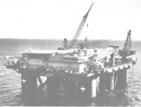
Semisubmersible, multi-service offshore rig SVV Safe Concordia was delivered recently by Gotaverken Arendal to Consafe Offshore.
