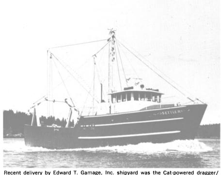
scalloper Settler, designed by Woodin & Marean, Inc. and constructed for Capt. Didrik Didriksen.
