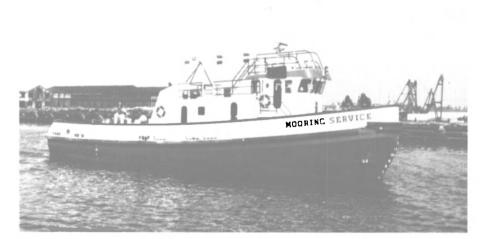
New mooring tug Mooring Service, built by Halter for Zapata Marine Service, has collapsible mast to facilitate line handling.
