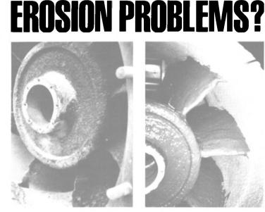
EROSION/CORROSION accelerated by impingement and entrainment nearly destroyed the guide vanes on this circulating water pump at a power plant in New Jersey. The guide vanes were quickly and economically rebuilt on site by the plant engineers using Belzona<sup>®</sup> Ceramic Metals, Belzona<sup>®</sup> Ceramic Metals can be used in every major fluid flow application where erosion/corrosion is your #1 enemy.
