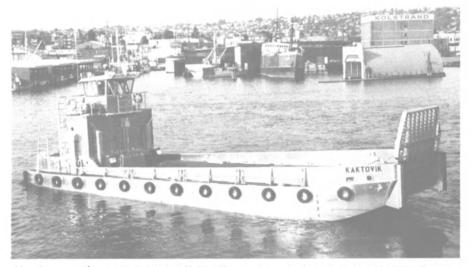
Aluminum self-propelled lighter Kaktovik was launched recently by MARCO Seattle. Built for Crowley Maritime, vessel is powered by three Detroit Diesel engines.
