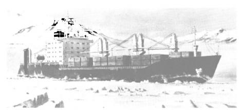
Artist's rendering of ice-breaking, multipurpose cargo vessel that Wartsila will build for Soviet Ministry of Shipping. Each of six ships will be powered by two Wartsila/ Sulzer 14 ZV 40/48 diesel engines with total output per ship of 21,000 bhp.
