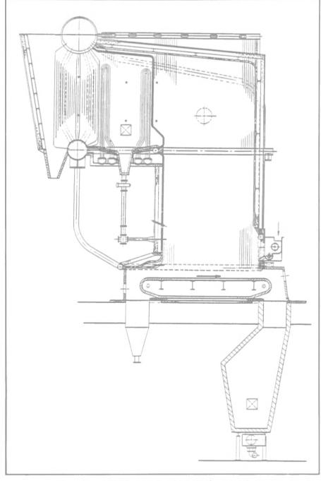
Figure 2 --- V2M9S spreader-stoker fired marine boiler.
