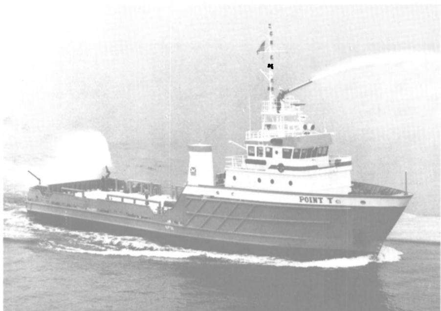
Fire/utility boat Point 'T', built by Halter Marine for Point Venture, Ltd., is first of a new line just introduced. Vessel is powered by two 900-bhp Detroit Diesel engines and fitted with a Bird-Johnson bow thruster.
