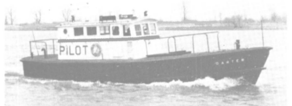
Pilot boat Darter is one of nine 48-foot vessels of this type designed and built by Dravo SteelShip for Panama Canal Commission.
