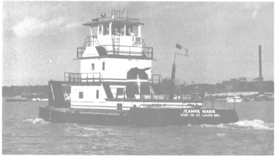
Marine Builders of Clarksville, Ind., built the Cummins-powered tugboat Jeanne Marie, and are completing work on two sister ships for Archway Fleeting and Harbor Service of St. Louis.
