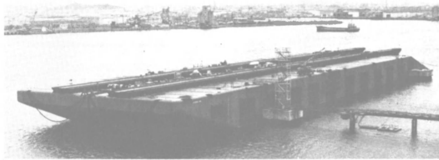
Largest of its kind in the world, 650-ft. Intermac 650, built by Hitachi Zosen's Sakai shipyard for McDermott Incorporated, is capable of carrying 36,300 metric tons.
