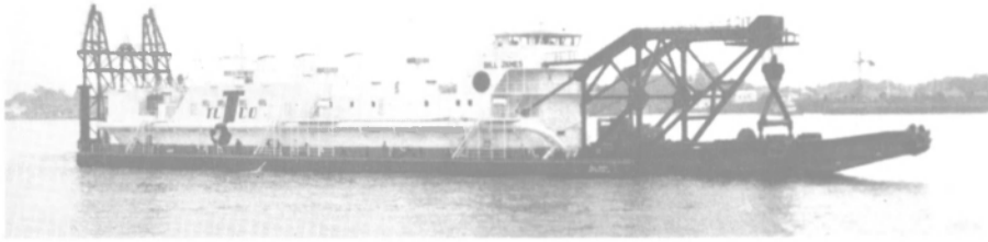
The 265-foot, cutter-suction dredge Bill James is the ninth vessel of its type to be placed in service by T.L. James Company of Ruston, La. Designed by naval architect Carlos A. Monje , dredge was built by Bergeron Industries, Braithwaite, La.
