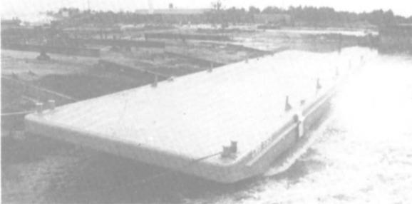
A significant event occurred recently at Bergeron Marine when the barge CMS-563 (shown above) slid down the launchways at the company's Port Bienville facility. The 120-foot by 30-foot by 7-foot steel deck barge built for Central Marine Service, Inc., New Orleans, was the 100th vessel constructed at the Mississippi yard.
