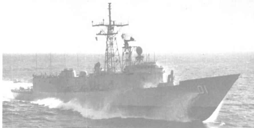
The HMAS Adelaide shown on sea trials on Puget Sound prior to recent delivery and commissioning. The General Electric gas-turbine-powered, guided-missile frigate is first of four being built by Todd Pacific Seattle for the Australian Navy.
