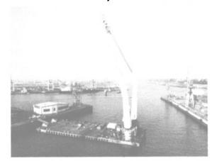
The 900-ton, heavy-duty floating derrick Tog Mor (shown above) was delivered re-cently by Blohm + Voss AG, Hamburg. Built for Howard Doris Ltd. of Edinburgh, the derrick's hull is 101.4 meters long and 27.4 meters wide (about 332.7 by 89.9 feet). It has been towed to Loch Kishorn yard in Scotland.
