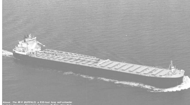
Above: The M/V BUFFALO, a 635-foot long self-unloader built for American Steamship Company. Buffalo, New York. Designed with an unloading rate of 3,500 short tons of coal per hour or 6.600 long tons of ore per hour, the M/V BUFFALO has a cargo deadweight of 23,110 long tons.
