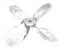
Starboard -7' diameter - pitch constant 4.699: Bore tapers from  $6\frac{1}{6}$ " to  $4\frac{53}{64}$ ".  $14\frac{1}{2}$ " taper equal to 1"/foot on diameter. U.S. Navy reconditioned. Average weight 1760 lbs.
