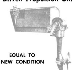
Equal-to-new-condition. Driven by GM 6-71 diesel—165 HP (a) 1800 RPM-2-cycle-6 cylinders. Weight 9300 lbs-48" X 24" propeller. Unit shown with outboard shaft in running position. Distance from deck to bottom of skeg 89". 4 Units immediately available.
