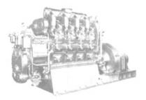
GM 8-cyl. engine — 8½ X10 — 2-cycle — Vee type driving 350 KW G.E. generator—440/3/60—600 RPM—430 KW 2 hours. 3 Units available. Your inspection invited.
