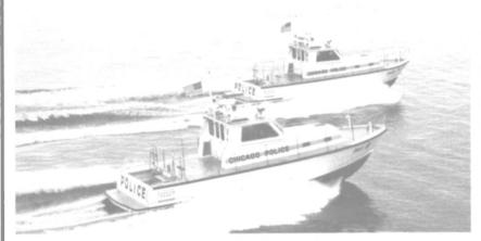
45' LOA Steel Hull Patrol Boats for Chicago P.D. - 600 HP - 25 MPH
