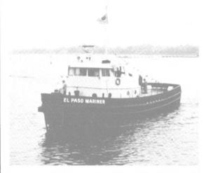
Passenger/Freight vessel by Blount Marine, 64'-6 X 21'-0 X 7'-4, Twin GM 8V-71N 460 HP EA, 3:1 Allison Reduction Gears, 42 X 28 Columbia Hydrosonic Props, Keel Coolers, 22.5 KW gens, 35 passengers plus one 20'-0 container (20,000 lb). Excellent Condition \$350,000
