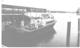
46' Crew Boat Aluminum Construction by Neuville Boat, 46' X 15' X 5' Twin GM 8V-71N 440 HP EA, 2:1 Reduction gear, 28 X 32 3 blade props, Keel Coolers, 7.5 KW gen, 30 passenger. Like New \$180,000
