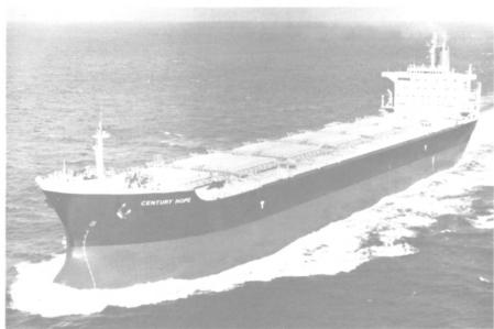
The 68,082-dwt bulk carrier Century Hope was recently delivered at the Tamano Works of MES to her owner, Kowin Shipping Company Limited of Hong Kong. Driven by a set of Mitsui-B&W 6L67GBE diesel engines' she recorded a maximum trial speed of 16.32 knots.
