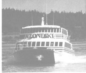
passengers, is powered by two Caterpillar 3412 TA main engines (Niigata 2.5:1 reverse reduction gear) and can reach a cruise speed of 28 knots. The hull and superstructure was specially designed by Nichols Brothers to allow for convenient landings on the banks of the Yukon where the vessel will cruise during 1985. Until then, after carrying passengers between Long Beach and Catalina Island during the Los Angeles Olympics, it moved to San Francisco for a season of dinner cruises
