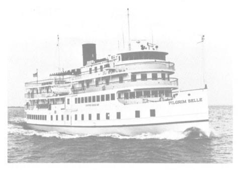
bhp at 1,800 rpm. Power is transmitted to the 4-bladed Columbian Bronze propellers through Twin Disc reduction gears. Shafting is 4inch Armco Aquamet; engine controls are by Kobelt. The bow thruster is a Schottel Model S-51, driven by a Detroit 3-71N diesel. Cruising speed is 15.7 knots.
