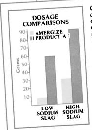
Graph shows quantities of AMERGIZE" deposit modifier/combustion improver and of a leading competitive product required to maintain low and high sodium vanadium slag in a dry state to a temperature of 1180°C. In low sodium slag, 12 X more competitive product was required, and in high sodium slag, 3 X more competitive product was required, than AMERGIZE.
