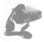
The RS-8000 is a fully synthesized radiotelephone with U.S. and international VHF channels and dual-watch, channel-16 priority with the capacity for all future channels when authorized.
