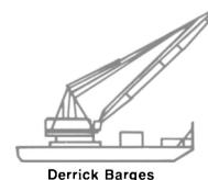
Derrick Barges 25 to 200 Tons Capacity
