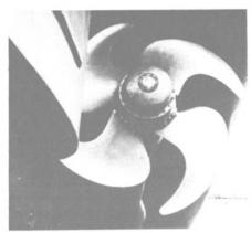
A modern highly skewed KaMeWa controllable-pitch propeller.
