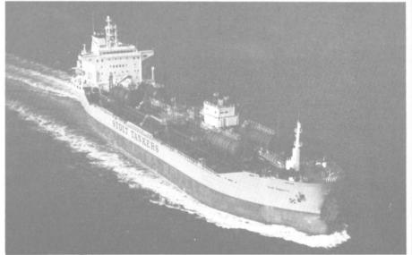
feet, depth to main deck of 49.2 feet, and design draft of 34.5 feet. Main propulsion is provided by a two-stroke Hyundai/B&W 6L60MC diesel engine with an output of 12,480 bhp at 111 rpm. Service speed is 15 knots at the design draft on a daily bunker consumption of 35.8 metric tons of heavy fuel oil, including full seaload on a 900-kw shaft generator.
