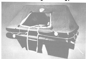
The six-person throw-overboard type commercial USCGapproved life raft from Viking has two individually inflatable buoyancy chambers, each of which has enough buoyancy to carry the weight of six people. For extra insulation, the raft has a double floor, which can be hand inflated.
