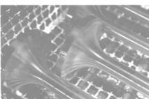
Each valve is checked for cracks by MWH. Crack detection testing includes the use of fluorescent penetrants.
