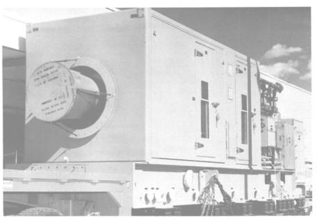
An Allison Gas Turbine generator set, model AG9130, such as the one shown, will provide all shipboard electrical power for the new Arleigh Burke Class destroyers.
