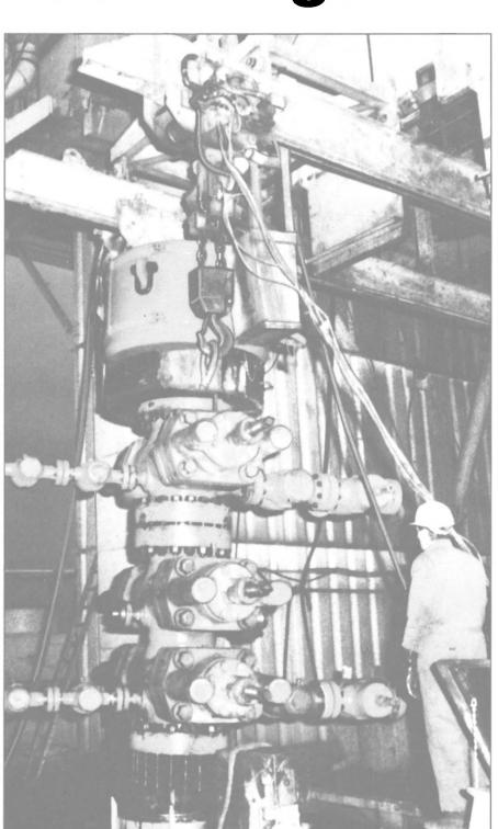
They are for instance standard built for application in areas where there is a risk of explosion. Explosion proof requirements are especially high on drill platforms. For this reason increased sparking protection is possible as an optional extra. JDN-pneumatic hoists are available with carrying capacities from 0,1 to 100 tons.
