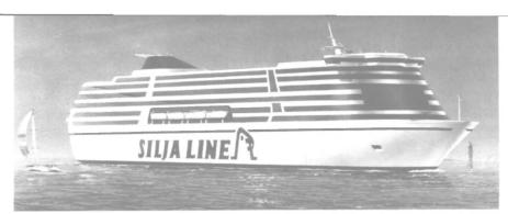
Artist's conception of the newbuilding for Silja Line. The vessel's machinery consists of four Wartsila Vasa 9R46 main engines and four Wartsila Vasa 6R32 auxiliary engines.
