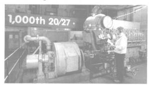
The 1,000th MAN B&W 20/27 engine recently underwent acceptance testing in the presence of the customer and representatives of the classification society. The engine is one of two 12V 20/27 engines (each developing 1,200 kw at 1,000 rpm) for the propulsion plant of a luxury yacht being built for an American owner by the Dutch yacht and shipbuilders C. van Lent & Zonen, La-Kaag.
