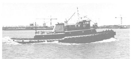
The 4,200-hp J.A. Bisso II is one of three oceangoing tugs E.N. Bisso and Son, Inc. is employing in its new long-distance towing activity. The tug is 125 feet in length with a beam of 29.6 feet. E.N. Bisso and Son operates 13 tugs in the New Orleans harbor.
