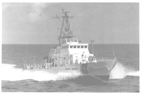
The USCG patrol boat Farallon, first of the Island Class built by Bollinger Machine Shop & Shipyard, is powered by two Paxman Valenta engines.
