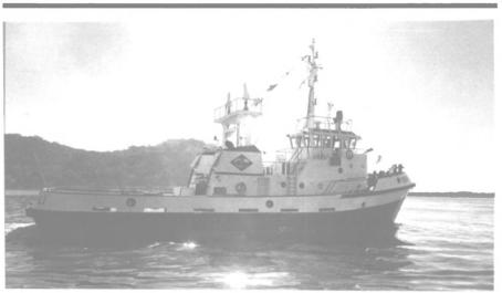
The Deutz MWM-powered Pemex L1 is the first of four harbor tugs being built for Mexico by Astilleros Unidos de Mazatlan.
