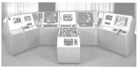
Radio Holland's Datamation is a complete integrated ship management system. One navigator can control and operate all the nautical and technical equipment on board.
