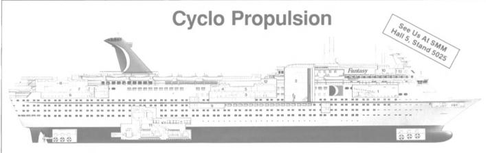
M/S FANTASY and M/S ECSTASY, cruise vessels constructed at MASA-Yards for Carnival Cruise Lines will each feature 2 x 14 MW CYCLO propulsion drives, 6.6 kV switchboards, four 10.3 MVA and two 6.8 MVA generators, plus six thruster motors and the main transformers, all engineered and supplied by ABB Marine, Helsinki.
