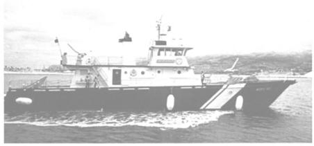
The Moku Ahi is a fully automated firefighting and rescue vessel manned by a crew of five. All engines and firefighting systems can be operated from the pilothouse.
