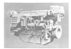
Dorman Sea King 8 marine diesel engine, part of the propulsion package recently installed in a Greek purse seiner.
