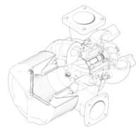
Cutaway drawing of the new RR 131 turbocharger from ABB Turbo Systems, which will be introduced in the spring of 1991.
