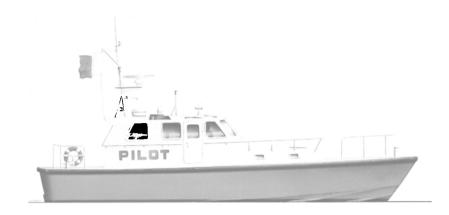
The new fiberglass hull design shares standard features unique to Gladding-Hearn pilot boats, including curved deckline and radiused transom corners for easy departure from ship side, wide 36-inch sidedecks, all-welded handrails inboard, and ship-grade windows, doors, piping and electrical systems.
