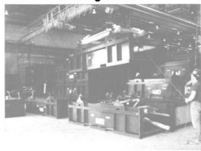
Material handling is simpler and safer at BIW with the new HF Cradle System from Dwight Foote, Inc. The designs of the container and self-aligning and interlocking cradle system create a one-piece unit that can be handled from the floor by one man using an overhead crane and an HF system spreader beam
