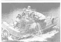
The first craft in the 47-foot rescue and patrol boat class successfully self-rights in 5.3 seconds during its recent rollover test at Textron Marine Systems in New Orleans, La.
