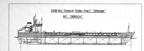
Outboard profile drawing of the Lindenau-designed double-hull chemical/oil tanker "Dorsch." She is equipped with 17 cargo tanks—12 side tanks and 5 center tanks—with a total capacity of 27,740 cubic meters.
