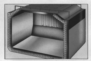
All structural reinforcement is located between the hulls. Therefore, the sides of the tanks or the holds are smooth and entirely free of sharp edges.
