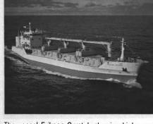
The vessel Erikson Crystal, showing high-speed Liebherr cranes of type CBW 5/19 Litronic, capable of working under offshore conditions.
