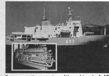
Four generating sets, two of them driven by 1,400-kw 14V 20/27 Bazan-MAN B&W engines (in the picture) and two by 7L 20/27 engines, are the prime movers for the diesel-electric propulsion plant of ocean research ship Hesperides.
