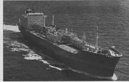
The cargo tanks on the Saulkrasti are designed for maximum pressure of 5.4 bar and 30 percent vacuum, and for a lowest transport temperature of -48 degrees C. The gas plant enables the ship to cool down, warm up or maintain all cargoes at any requested working temperature. With a total pump capacity of 1,500 cubic meters an hour, time of discharge is about 10 hours.
