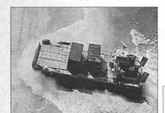
Built by Textron Marine Systems, LACV-30s accommodate a wide variety of payloads and can be disassembled for transport by truck, rail, aircraft or ship.
