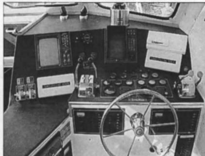
All electronic displays, switch panels, navigation aids and vessel controls are built into this circular console.
