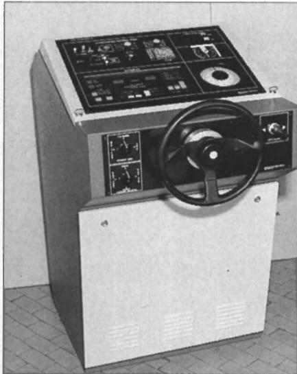
A sliding drawer inside the Nautamaster steering control stand allows mounting of the Polaris MK2 gyrocompass, thus providing easy access for maintenance and service operations; incorporated in the upper steering console plate of the Nautamaster is the control panel of the gyrocompass equipment.
