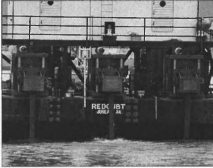
Three 255-hp Model OD250 Thrustmaster steerable propulsion units were recently installed on an Alaskan transport barge.
