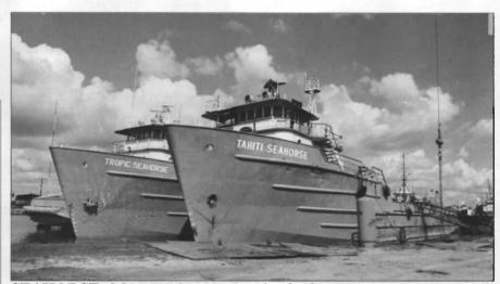
SEAHORSE CONVERSION—Besides building the Spirit of Norfolk, Service Marine also has three 176-foot supply oilfield vessels under repair and conversion. The ex-Tahiti Seahorse, soon to be the F/V Arctic Quest, will be converted for Arctic Quest, Inc., Homer, Alaska, and will join the crab fishing fleet near Dutch Harbor. The vessel will feature complete equipment renovation and a new Caterpillar engine and generator package furnished by N.C. Power Systems of Seattle.
