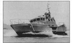
The U.S. Coast Guard's 47-foot motor lifeboat has a maximum operating speed of 28 knots and an associated range of 220 nautical miles. The hull is lightweight yet strong enough to withstand hurricane force winds and 20-foot breaking waves. The boat has the capability of a complete rollover and can self-right in 30 seconds or less.
