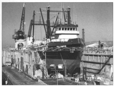
Photo shows Marine Industries Northwest Inc.'s new drydock, MINI I, with Western Pioneer freighter Yellowfin docked for a scheduled underwater inspection, tailshafting repairs, and painting.
