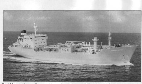
The LPG tanker Norgas Energy which was fitted with a new Wartsila Vasa 7R46 main engine.
