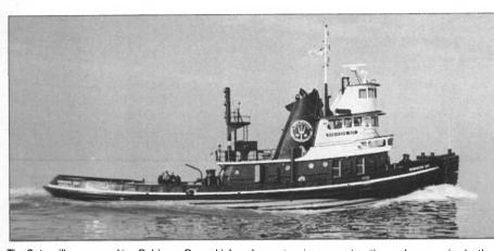
The Caterpillar-powered tug Robinson Bay, which underwent major reconstruction and repowering by the Shipyard Division of The Great Lakes Towing Company in Cleveland, will be used by the Saint Lawrence Seaway Development Corporation for buoy maintenance, docking assistance, salvage operations, and emergency replacement of lock gates.
