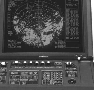
On-screen data readouts include range, bearing, course, speed, CPA, TCPA, BCR (bow crossing range), and BCT for up to 3 selected targets, as well as own ship course and speed.
