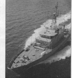
The two new patrol boats built by Moss Point Marine for the Ecuadorean Coast Guard are equipped with armament foundations for one 40mm cannon and two 50-caliber machine guns. The new "Espada" class Trinity design can accommodate a variety of weapons suites, depending on the mission of the boat.
