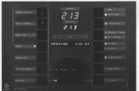
Besides indicating the actual position on a sea chart, the NAUTOPILOT offers, in systemtechnical combination with the adaptive autopilot NAUTOPILOT A, the track controller NAUTOTRACK and
