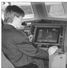
The navigation system NCIS 1800 from Krupp Atlas Elektronik offers the user versatile decision-making aids for navigation. It performs monitoring and advisory functions, ensuring high operational safety of the ship.
