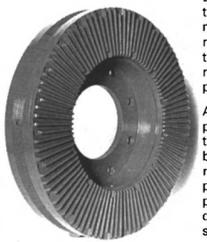
Aluminum alloy ribbed housings of robust design provide cooler operation with less variance between cold and hot performance. Dampers are bolted construction and are serviceable with factory rebuild program. LO-REZ forced-damped computer program handles very large and complex power trains and provides for optimization of damper size and characteristics. Standard damper sizes are available as well as custom-engineered models.
