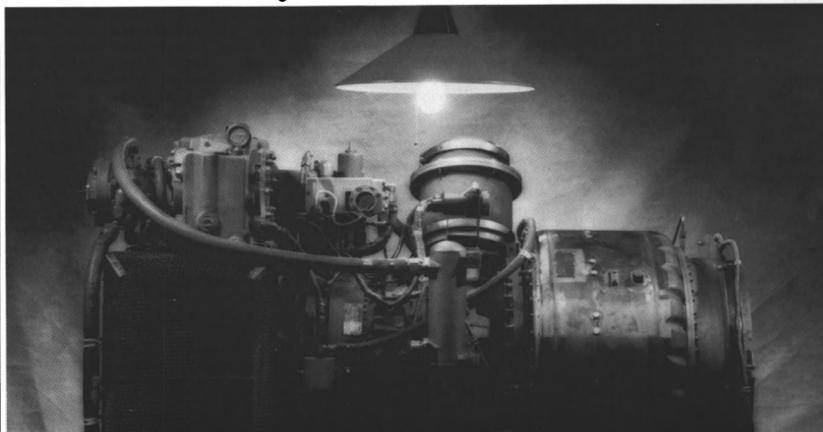
*The TF40. Only 4,000-shp class marine turbine to be Navy-certified for shipboard propulsion.*
