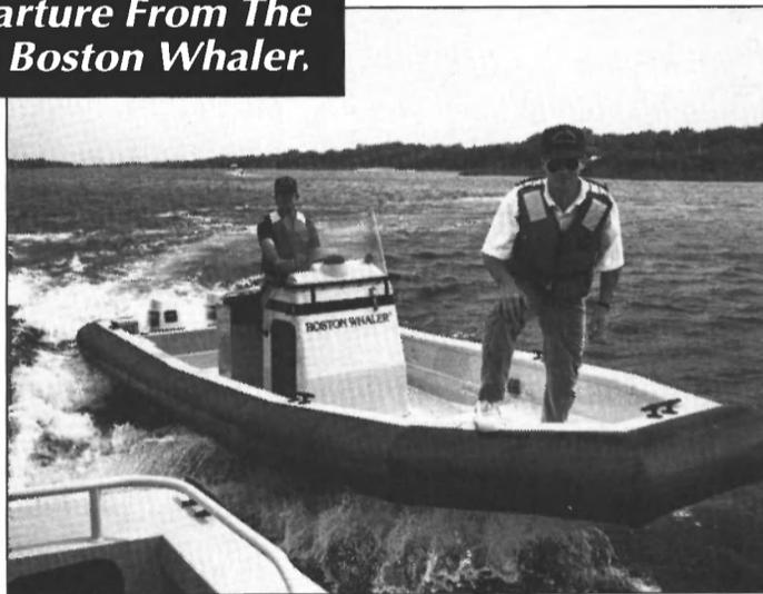
Impact 21' combines the unsinkable, virtually indestructible Boston Whaler foam cored hull with a fully fitted foam collar. This unique fendering system provides full time protection against punctures and abuse of all kinds, and will not deflate. Step into the new world of soft-sided boats. Impact 21' by Boston Whaler.
