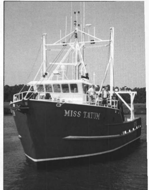
Stern Dragger built by LaForce Shipyard.
