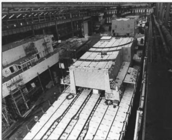
Yarrow Shipbuilder's warship/frigate being externally protected with MegaFilm.
