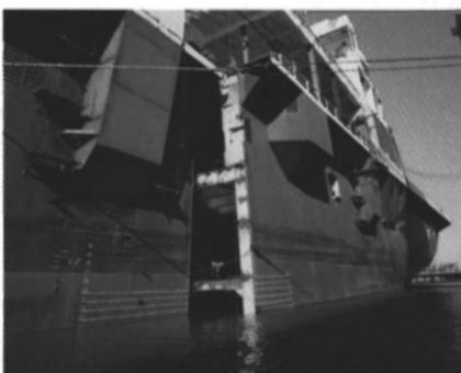
Consider the S. S. Northern Lights, we lengthened the ship from 700 feet to 790 feet increasing the cargo capacity by 40%. Then we passed stringent ABS and U.S.
