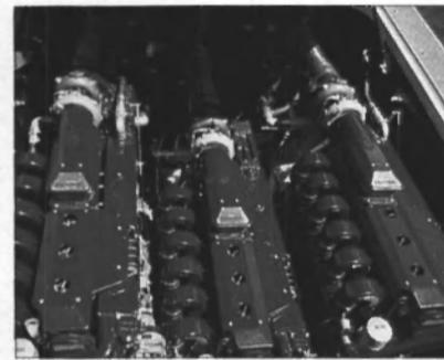
Three Seatek six-cylinder in-line models are placed side-by-side in the patrol boat's narrow, performance hull.
