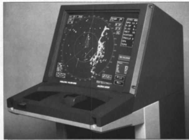
Other standard features include interswitching, dual preset Guard Zones; the NAVCARD for extended, customized map creation, storage, and retrieval; and an improved plotting facility. The ARPA also features a simulator for training and maintenance tasks.
