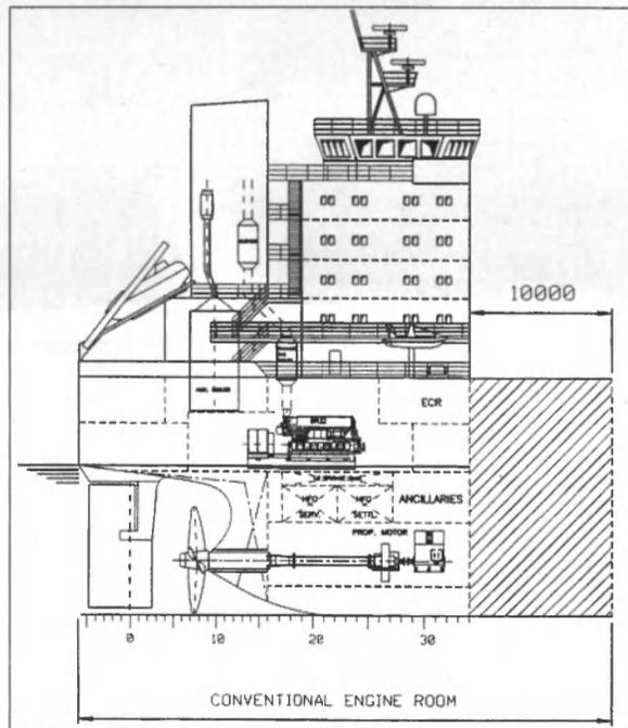
Fig. 2: Savings in engine room length (and gain for cargo space) is made possible by a modern diesel-electric plant.
