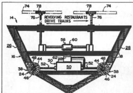
Cutaway of the hydro-propelled ship.
