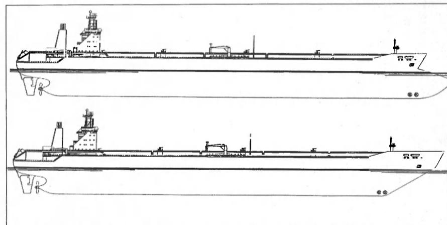
Kvaerner Masa-Yard's new 120,000-dwt arctic tanker design is available with a bulbous bow or in an icebreaking version.
