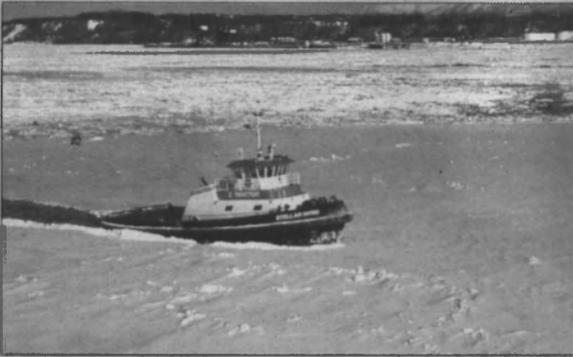
The 85-foot (25.9 m) tug *Stellar Wind* cuts through the ice in Cook Inlet, Alaska on its way to a late-winter ship-assist assignment. The 3,000-hp vessel was designed and built to Ice Class 1-C requirements for Cook Inlet Tug & Barge by Tri-Star Marine of Seattle. The yard is currently building a similar tug, the 85-foot *Tioga*, for Coos Bay Towboat Co. of Ore.
