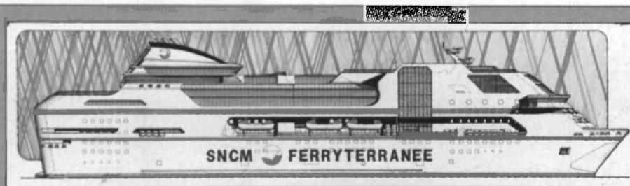
This new car ferry—to be built by Chantiers de l'Atlantique—will be powered to a 23.8-knot service speed by four diesel engines.
