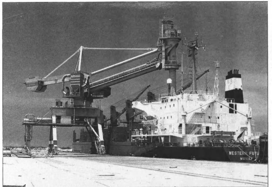
Continuous ship unloader by PWH Anlagen, a company of Krupp Fordertechnik.
