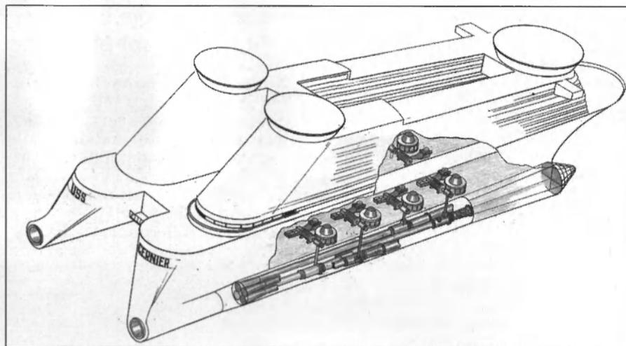
The recently patented hydro-propelled ship would require a 25,000-hp powerplant. The inventor is currently seeking a builder for the vessel.
