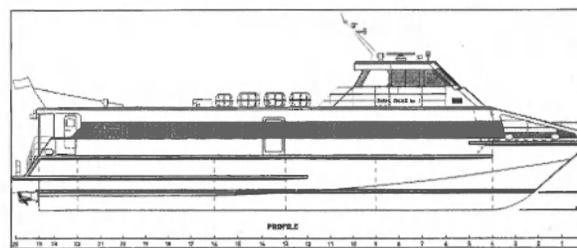
Profile drawing of a 98-foot (30-m) monohull passenger vessel, two of which Yuet Hing Marine Supplies Company ordered from Austal Ships.
