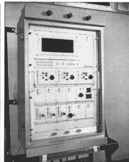
DGM4 degaussing system was used on Intermarine's Osprey minehunter to achieve an extremely low magnetic signature.
