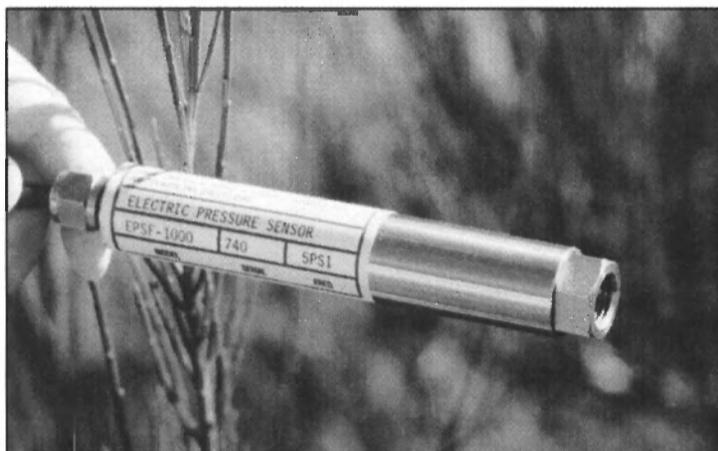
*PRESSURE SENSORS are installed overhead in the engine room of the VICTORIA CLIPPER. Tubing connects the sensors to the monitored locations. Two sensors check raw water (engine coolant) and one reads oil pressure. Individual sensor (above) has a frequency output to eliminate electrical interference.*
