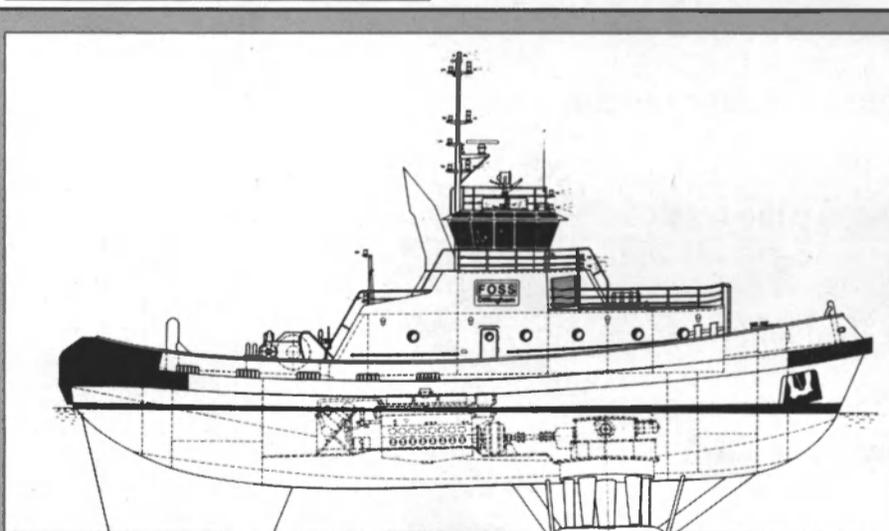
Pictured is a diagram of a tractor tug with Voith-Schneider cycloidal propulsion. The Voith-Schneider tractor tug configuration entails specific features, including:
