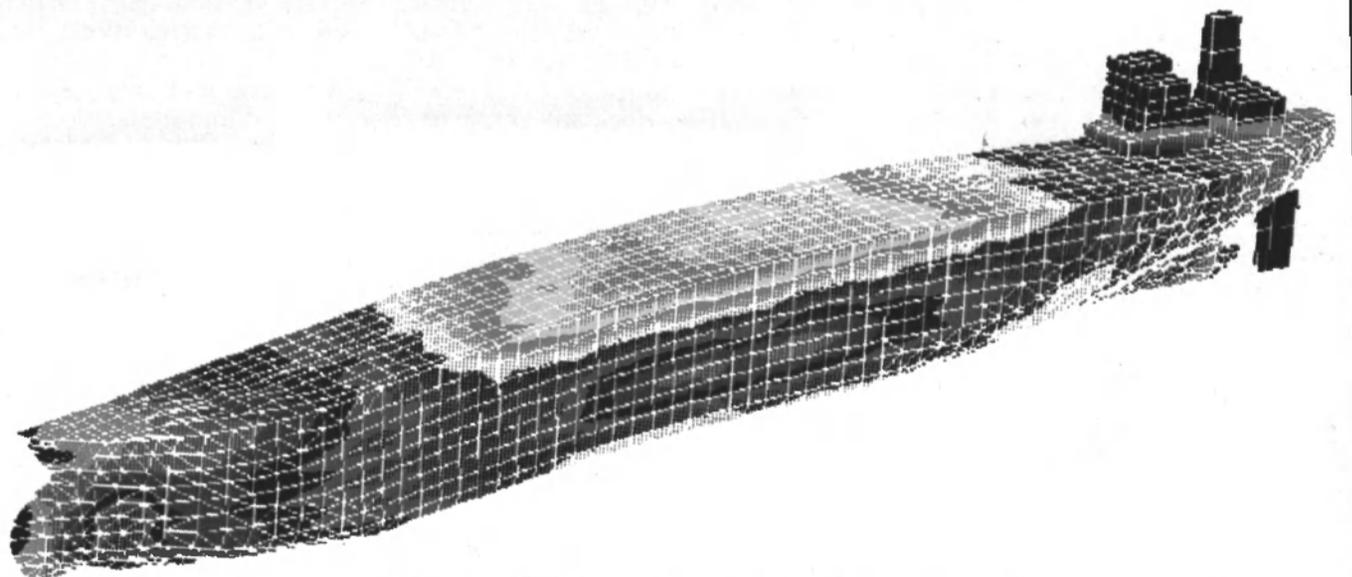
Color stress plot of forces acting on a VLCC causing a hogging condition.
