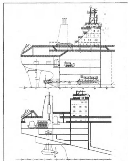
The new tanker design also has a propulsion arrangement option—incorporating either a pair of diesel engines (top) or an Azipod propulsion unit (bottom).
