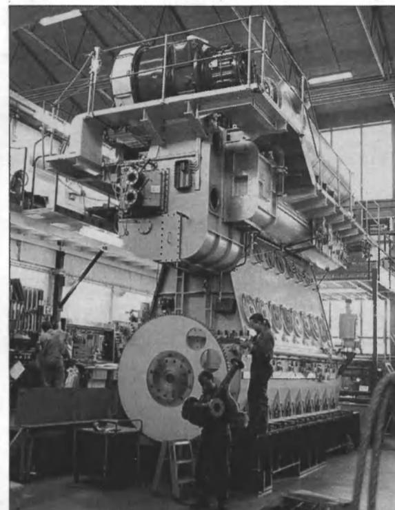
Assembly of the first 8S35MC engine.
