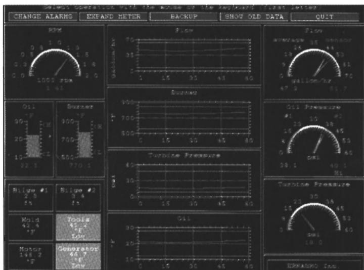
*MAIN SCREEN shown in CHANGE ALARM condition allows setting Hi-Lo alarms over full range of any selected function. Besides providing electrical signals for audible/visual signals, alarms are indicated in red on screen.*
