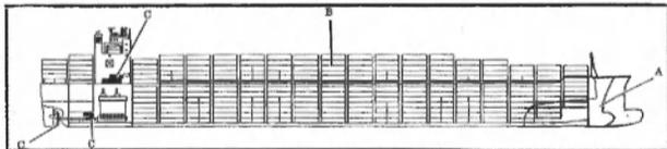
ACV conversion to SL31. Work includes forebody modification (A), midbody removal (B) and shaft motor & generator (C).
