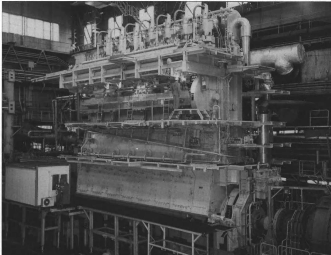
Fig. 1: A Sulzer 7RTA84T engine of 36,960bhp (27,160kW) at 74 rpm. The first of its type, it was built by Diesel United in Japan and is being installed in a 258,000-dwt NYK tanker.
