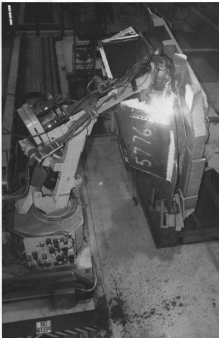
CYBO Robots helped modernize General Dynamics' Land Systems Div.'s Lima, Ohio plant with robotic welding stations to build the M1A1 Abrams battle tanks more efficiently. The company is currently working—with the help of the government and shipbuilders—to develop portable shipbuilding robotics to help make the U.S. competitive on an international level.
