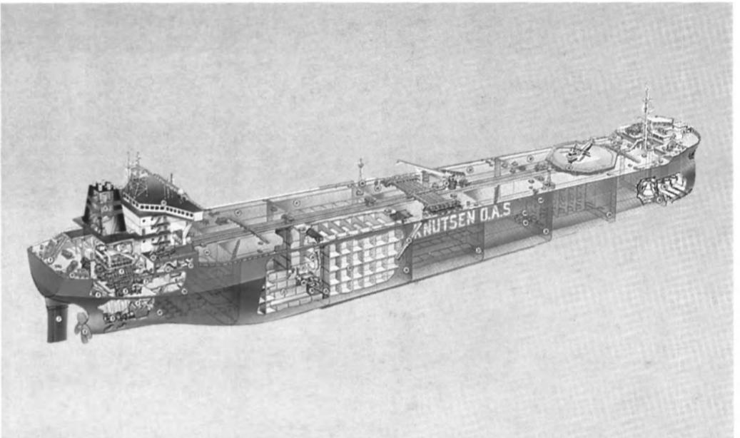
Diesel-electric advanced 125.000 DWT shuttle tanker.
