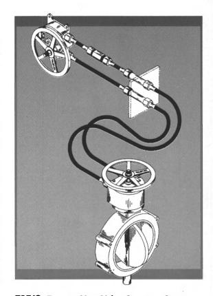
**RVVO:** Remote Vent Valve Operator Systems are lightweight, low-profile operators that bolt directly to flanges of 1/4-turn ventilation valves. Systems incorporate a patented override feature at the valve for local operation.
