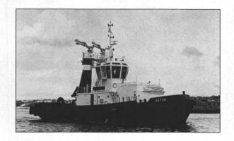
Astilleros Zamacona, member of the Construnaves group of shipyards, made the first two deliveries of an order for four multi-purpose Voith tractor tugs to Spanish towage company Cia. de Remolcadores Íbaizabal. These supertugs are fitted with Voith-Schneider water tractors driven by two 1,930-bhp Wartsila Diesel
