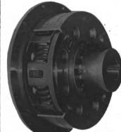
LO-REZ helical steel-spring couplings, with their low, constant and accurately-controlled torsional stiffness factors, provide excellent torsional characteristics for geared marine reciprocating propulsion systems, engine and reciprocating compressor drives of many varieties, locomotive drives, etc.
