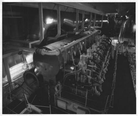
HDW says this slow-speed, two-stroke diesel, Mitsubishi 7UEC85 LSC engine plant installed on its Not Fribourg open-top containership driving a fixed-pitch propeller is economical, reliable and easy to mai The engine has a nominal output of 27,290 kW (37,100 hp) with 102 min -1 rpm and a low specific consumption of 165 g/k Wh (121 h/hp).
