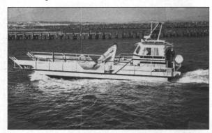
Cleansea Bravo 120 Oil Spill Response Vessel built by Marshall Branson Marine, commissioned by Caltex Services Ltd.
