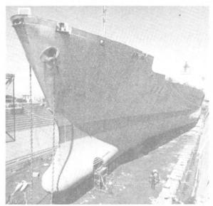
"LOW AND DRY" in graving dock at Triple A Shipyard in San Francisco, Matson Navigation Company's container-RO/RO carrier Lurline is undergoing extensive work that will improve her fuel efficiency and expand cargo capacity. During six-week shipyard stay, the 862-foot vessel's underwater hull exterior will get coats of International Paint Company's self-polishing copolymer bottom coating that repels marine growth and is another fuel saver.
