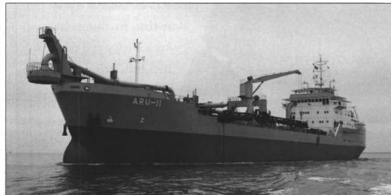
Hopper suction dredger *Aru II* is one of two nearly identical vessels delivered to a state-owned Indonesian enterprise by Krupp Fordertechnik. A cutterhead suction dredger, *Batang Anai*, is scheduled for delivery to the same customer this fall.
