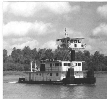
The towboat *Bettendorf* (left) and the nearly identical *Fred Lee* (above), were recently delivered by Trinity's Equitable Shipyards to the U.S. Army Corps of Engineers. The only difference between the two vessels is that the *Fred Lee* has a hydraulically-operated elevated pilot house which can rise 10 ft. (3 m) above the waterline.
