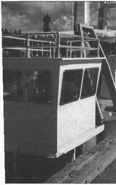
Carolina Cockpit of Portland, Ore. supplies government and commercial marine operators with ready-to-install, corrosion-proof, engineered deck structures and control cabs. The first of five five-ft. by seven-ft. (1.5- to 2-m) upper pilothouses was delivered recently to the Panama Canal Commission. These houses have tempered glass aluminum framed windows, roof access ladders, removable
