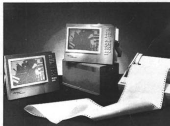
CHART VIEWER is built to the following Mil Spec specifications: Water Resistance and Salt Exposure MIL-T 28800c paragraph 4.5 6.2 Vibration 1.5g 10-100H Shock 5 G peak.
