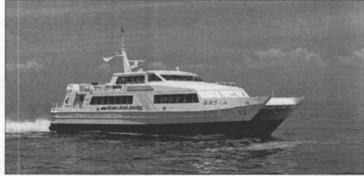
Hitachi Zosen completed the *Apollon*, a foil-assisted catamaran in its Superjet-30 series, at its Kanagawa Works and delivered the vessel to its owner, Fuke Kaiun Co., Ltd. in Osaka. The vessel, the last of seven constructed consecutively by Hitachi Zosen, was commissioned in
