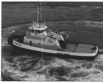
Tri-Star Marine of Seattle delivered a 4,000-hp tractor tug, *Tioga*, to Coos Bay Towboat Co. of Oregon. The new 85-ft. (26-m), ice-strengthened boat was designed and built by Tri-Star, with engineering services by Jensen Maritime Consultants.
