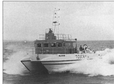
Twin Volvo Penta TAMD 122D turbocharged and aftercooled diesels provide the propulsion power for *Recover*. *Recover* is the Protector 54-based oil spill recovery vessel (OSRV) completed by Prout Catamarans for Thames Oil Spill Clearance Association (TOSCA), and operated on its behalf by the Port of London Authority (PLA).
