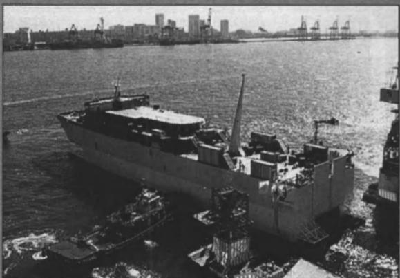
Kawasaki Heavy Industries Inc. launched a wave-piercing catamaran aluminum high speed car ferry, type Kawasaki Jet Piercer AMD 1500 Mark II for joint owners Maritime Credit Corporation of Japan, Tokyo and Kyushi Ferry Boat Co., Ltd., Yawatahama, Ehime Prefecture. The vessel is based on a design from Advanced
