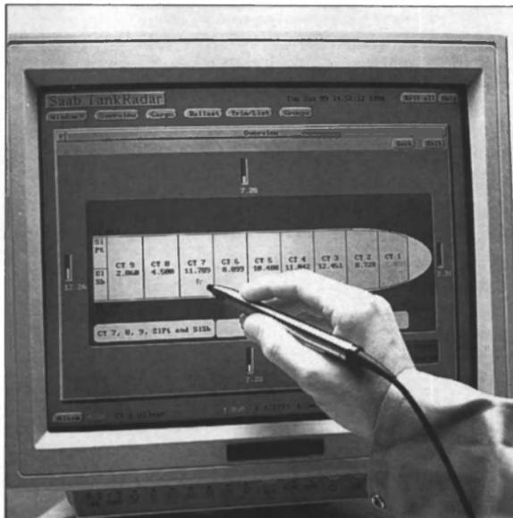
Saab has introduced a third generation of its TankRadar level gauging system, which uses a light pen to activate the system's various functions.
