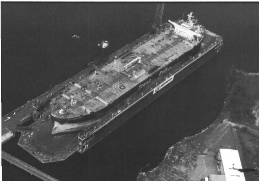
The two and a half year old *Stena Concertina* was in **Norfolk Shipbuilding and Drydock Corp.'s (Norshipco) Titan** drydock for blasting and coating; tailshaft and rudder clearance inspections; valve, pump and generator repairs; and other planned maintenance and inspections. The vessel is a technologically advanced double-hull oil tanker from Mitsui O.S.K. Lines.
