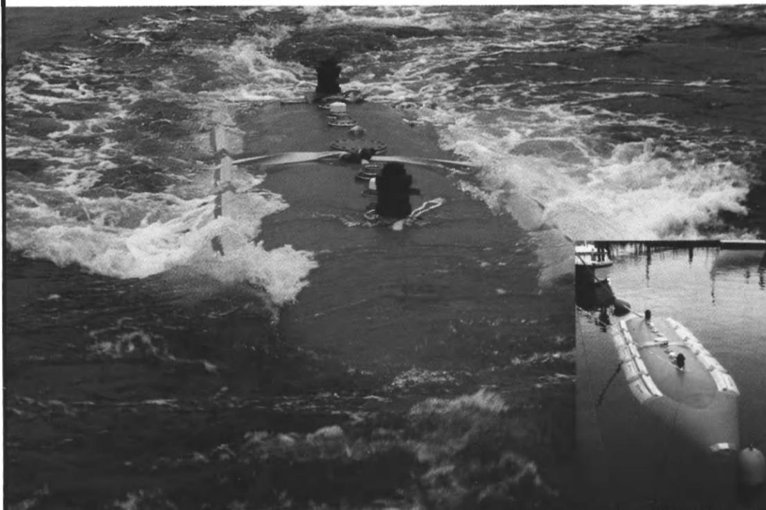
CANFLEX (USA), Inc.'s new 12,500-gallon Sea Slug under tow at approximately 5 knots during recent sea trials in Anacortes, Washington. Insert shows the unit moored alongside the dock, ready to be offloaded. The Sea Slug is an ideal unit for emergency lightering.
