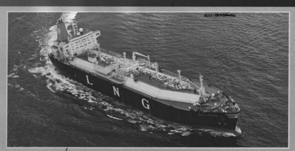
ops 28,000 shp at 83 rpm, driving a single screw through doulle reduction gearing, providing a service speed of 19 knots. Two water boilers produce 50,000 kg/h of super-heated steam
