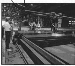
The ESAB retrofit included installation of a Series 2000 Control and a PT-15XL nitrogen/oxygen plasma torch with a height sensing mechanism.
