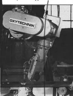
The Oxytechnik plasma system can cut plates up to 65 mm in thickness, and is equipped with a special design that allows cutting closer to the flanges.
