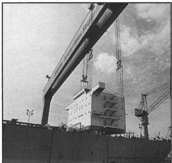
Pictured is the installation of the deckhouse on Double Eagle tanker *Despotico* at Newport News Shipbuilding.
