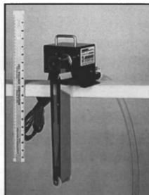
The Mighty Mini, manufactured by Abanaki Corporation, reportedly removes medium weight oil at a rate of two gallons per hour.
