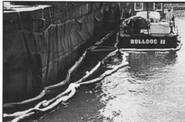
RIP WRAP protects the dock landing and vessel *Bulldog II* from the effects of re-oiling.
