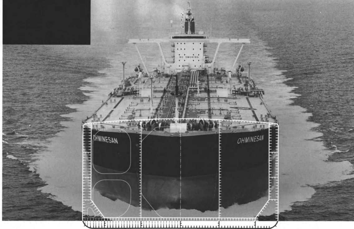
The *Ohminesan* is the fourth double-hull VLCC built by Hitachi Zosen.
