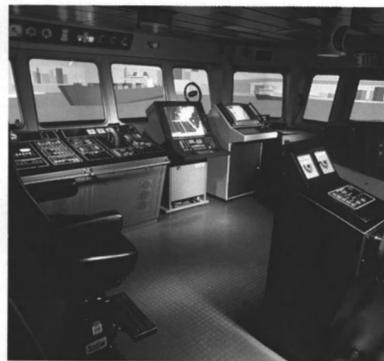
The interior of the Centre's Full Mission Ship Bridge Simulator, with full motion and 360 degrees horizontal field of view.
