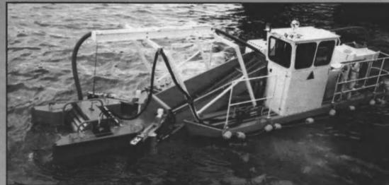
This "combo" oil/debris Marineskimmer offers rapid response to typical non-catastrophic, protected water oil spills commonplace in harbors, rivers and navigable waterways.
