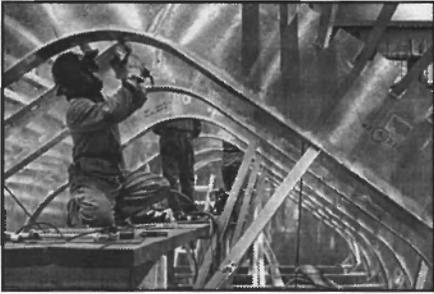
CFI employees are shown welding the first hull module of a high-speed aluminum ferry with ESAB welding equipment and filler metals.
