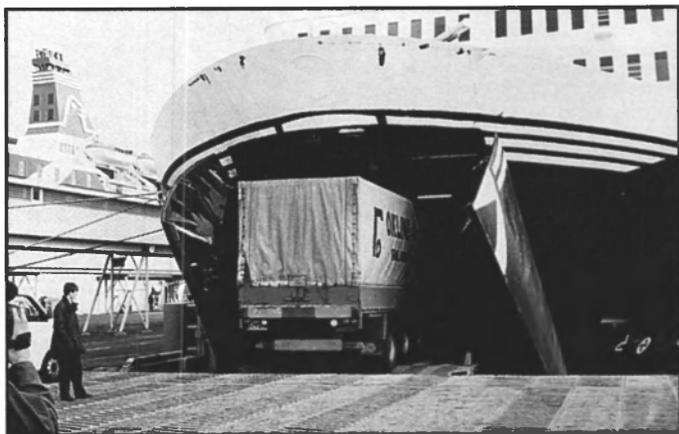
to avoid the inconvenience and delays of stern-only operation. It was at this time that MacGregor entered the picture, and the decision was made to adopt a completely different concept, with side-hinged bow doors.
