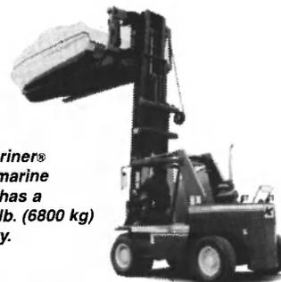
The Mariner® F1500 marine forklift has a 15,000 lb. (6800 kg) capacity.
