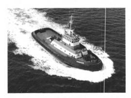
The tractor tug NAMAHOE, now in service in Hawaii; 4,400 HP with twin Z-drives: 105'  $\times$  34'  $\times$  16.5' (32  $\times$  10.4  $\times$  5m).
