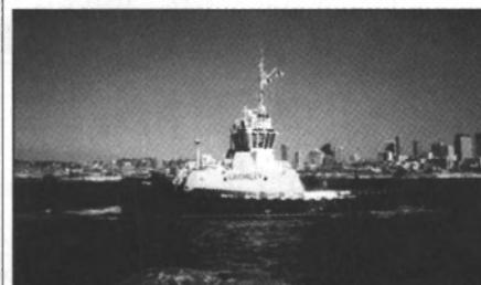
powered by two Caterpillar 3516-B engines and has an indirect bollard pull in excess of 120 tons at 10 knots. *Guide* was built by Nichols Bros. Boat Builders in Freeland, Wash.
