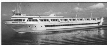
The ship's hull is steel constructed with an aluminum superstructure. It is powered by two D2842LE Man diesel engines, producing 1,440 bhp @ 1,800 rpm. The engines turn two five-blade 48 x 39 in. propellers, through Twin Disc MG-5202 gears, with a 2.92:2 reduction, achieving a service speed of 10 knots.
