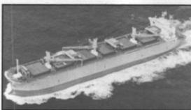
Forest Princess, a 51,152-dwt woodchip carrier ordered by Rioship Co. Ltd. was recently completed at the Maizuru Works of Hitachi Zosen. The vessel, under Panamanian registry, was delivered to the owner in late November. With an overall length of less than 656 ft. (200 m), Forest Princess can pass through the Inland Sea of Japan even at night. The vessel is equipped with a chip unloader composed of a hopper, deck cranes and conveyors for discharging woodchips to shore.
