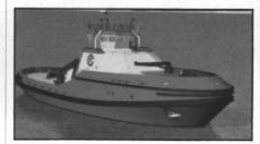
Caterpillar was chosen to power two new construction 10,192 bhp (7,600 bkW) tractor tugs for Vessel Management Services (VMS), a subsidiary of Crowley Maritime Corp., San Francisco. The 153 ft. (46.7 m) vessels are touted as being the most powerful cycloidal propulsion tractor tugs in the world. The vessels are being built at Dakota Creek Industries, in Anacortes, Wash., to provide
