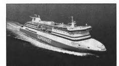
In early 1998, Kvaerner Masa-Yards' Turku New Shipyard delivered two fast vehicle-passenger ferries to Attica Enterprises S.A. for use in the Patras, Greece to Ancona, Italy route. The ferries are designed to maintain a regular 48-hour round trip with a service speed of 28.5 knots.
