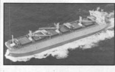
Forest Princess, a 51,152-dwt woodchip carrier ordered by Rioship Co. Ltd. was recently completed at the Maizuru Works of Hitachi Zosen. The vessel, under Panamanian registry, was delivered to the owner in late November. With an overall length of less than 656 ft. (200 m), Forest Princess can pass through the Inland Sea of Japan even at night. The vessel is equipped with a chip unloader composed of a hopper, deck cranes and conveyors for discharging woodchips to shore.
