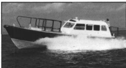
minum by Winninghoff Boats, Inc. Designed by Bill Preston of Marine Design, Inc., this boat is an updated version of a pilot boat design that Preston has been perfecting since 1976, incorporating improvements in equipment, systems and construction methods along the way. The most significant changes on this 1998 version are the use of foam fendering, the addition of a second helm station and the creation of NC cutting files for hull and superstructure components.
