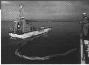
Authority (PLA) and the oil industry to provide a fast response to oil spills in the tidal Thames. TOSCA has a fleet of craft which are designed to cope with oil spills of up to 50 tons. One of the latest TOSCA vessels is Respond, built by RTK Marine.
