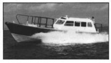
minum by Winninghoff Boats, Inc. Designed by Bill Preston of Marine Design, Inc., this boat is an updated version of a pilot boat design that Preston has been perfecting since 1976, incorporating improvements in equipment, systems and construction methods along the way. The most significant changes on this 1998 version are the use of foam fendering, the addition of a second helm station and the creation of NC cutting files for hull and superstructure components.
