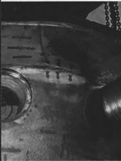
The Great Lakes ore carrier Herbert C. Jackson suffered severe damage — four ft. cracks — to its propeller hub. The hub was restored to original specifications using metal stitching.
