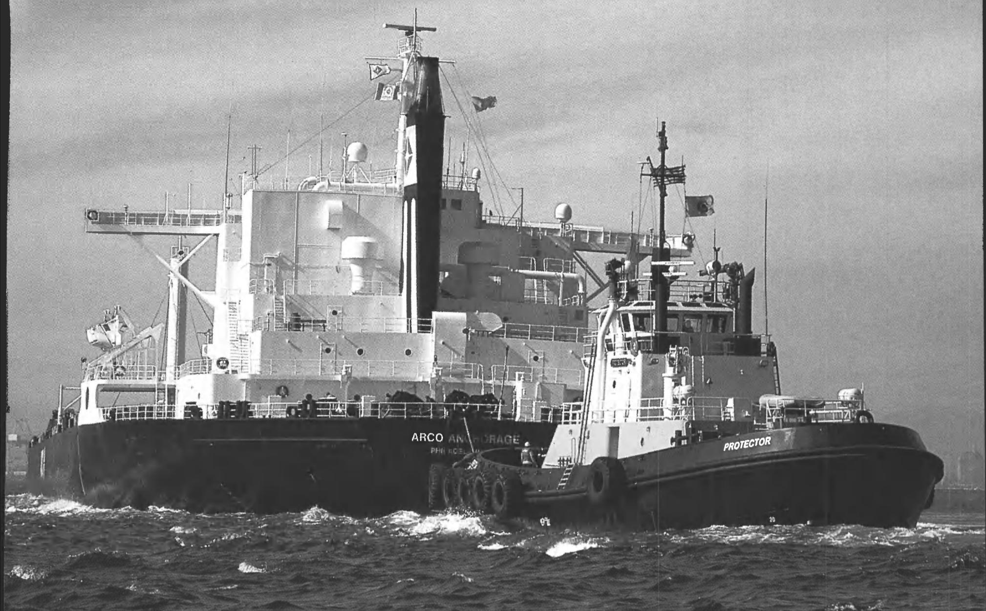
120 feet. 5,500 BHP. Voith Schneider twin cycloidal propulsion. Hydrofoil-shaped skeg. 300,000 pounds of indirect pull at 12 knots. More than just another answer – it's the solution.
