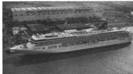
Following extensive dock trials, the 76,880-gt cruise vessel, Superstar Virgo left the covered building dock of Papenburg, Germany's Meyer Werff Shipyard. Built for Asian-based shipping company Star Cruises, the ship was towed out to a fitting-quay to complete the remainder of its interior design.
