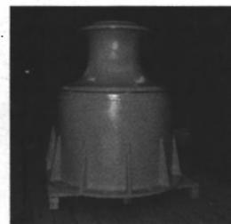
running pull at 35 fpm. Schoellhorn-Albrecht capstans are constructed to withstand severe operating conditions with minimum maintenance. Units are single or variable speed, with a choice of electric, hydraulic, pneumatic or manual prime movers. Electrical powered capstans feature marine duty "Crane & Hoist" design D motors for smooth starting under load, and 300 percent starting torque. Capstan options include special marine coating and explosion proofing for hazardous areas.
