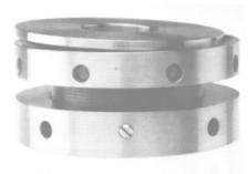
Vibracon SM elements, the universal adjustable chocks, are reportedly gaining in popularity for the mounting and chocking of machinery such as diesel engines, turbines, gearboxes, compressors, generators, E-motors and bearings. Patented by Machine Support BV of the Netherlands, the product is designed to permit quick and accurate alignment, in many cases eliminating the machining of foundations or base frames. The element is approved by Germanischer Lloyd, as well as by Navsea.
