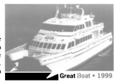
Phil Hercus of International Catamaran Designs Sydney, Australia, designed Yankee Freedom II. The Incat design uses a single chine Z-Bow hull shape that increases waterline length for improved high-speed performance and seakeeping ability.
