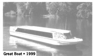
mum air draft of 6 ft. unique among the passenger vessel industry. Despite this low air draft, the interior is exceptionally luxurious for a scheduled commuter service liner. Able to accommodate up to 46 passengers, the vessels boast Boeing 737 reclining seats. Additional amenities
