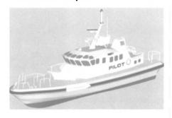
Kvichak Marine Industries has been granted the contract to build a 72 ft. (22 m) all-aluminum pilot boat for the Columbia River Bar Pilots Association of Astoria, Ore. Named Chinook, the vessel was designed by Camarc, Ltd. It is scheduled for an August 2000 delivery. Chinook is designed to survive a 360-degree rollover while maintaining a safe return to its mooring with crew and equipment intact.
