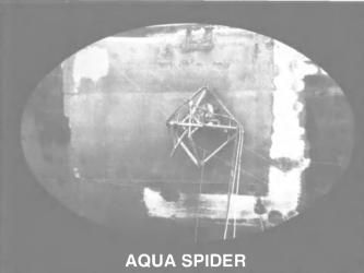
Removes paint and coatings from vertical surfaces with vacuum attachment for debris and water containment
