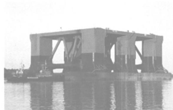
The multi-purpose bare-deck platform CS50 represents the fifth generation of semi-submersible platforms designed by Moss Maritime AS (Norway). The platform, which measures 389 x 231 x 133 ft. (118.6 x 70.4 x 40.6 m) with a hull weight of approximately 15,000 tons, is of a catamaran type with two pontoons and six stabilizing columns supporting the upper structure.
